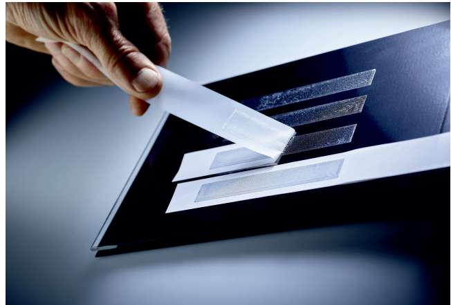
Fig. 2. Peeling off a strip as a quick test proves that the adhesive test strips adhere excellently to the ABS base plate © Arburg
